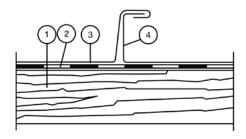
Fig. 2: Angular standing seam
