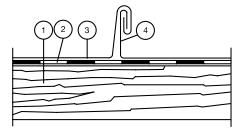
Fig. 1: Double standing seam
