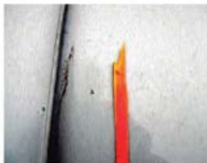
Wood chips and splinters absorb moisture, and can stay humid for enough time to mark the bright zinc surface. Care should also be taken with eZinc Allim®, Rainbow and Advance.
