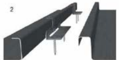
Clipped undercloak and the overcloak
