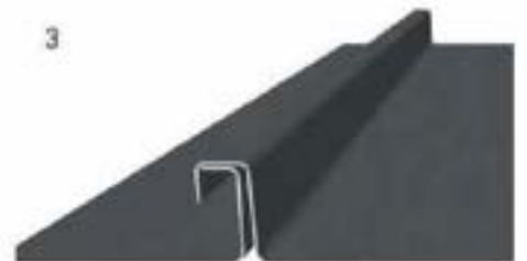
Small gap at base forms automatically and allows for lateral thermal expansion
