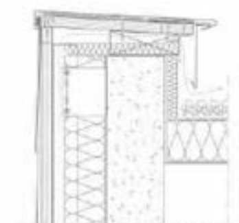
Rear vented capping (Rhomboid tile)
