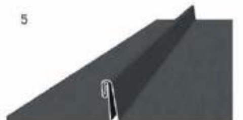
Double lock well, second turn completes double lock standing seam joint
