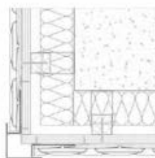
External corner (fish scale tile)
