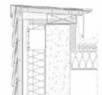
Rear vented capping (fish scale tile)
