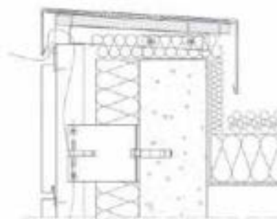
Front vented capping
