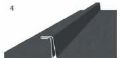
First turn completes angle standing seam joint
