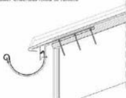
Gutter brackets fixed to rafters
