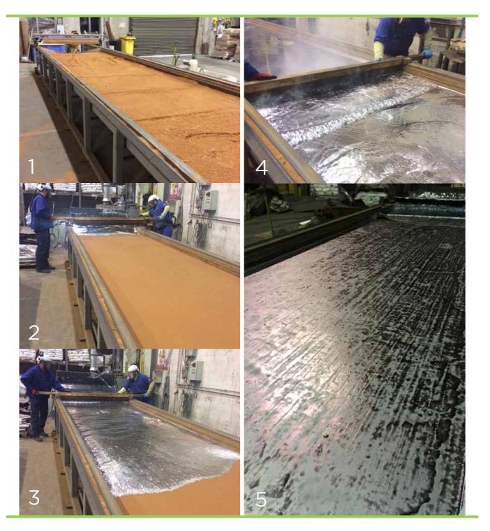
Sand cast lead is produced by pouring molten lead onto a bed of moulding sand; this process has been used for hundreds of years. Skilled operatives will then use a strickle to chase the lead to the desired thickness. Once it has solidified, it is then cut to width and length then rolled. Sand cast lead is available in standard codes of 6, 7 & 8 (other codes are available) and because it is produced to the specific sizes required, there is nominal waste.
