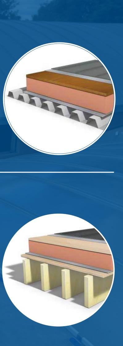
WARMFAST<sup>©</sup> removes the requirement for ventilated timber on the cold side using fewer materials and labour.
